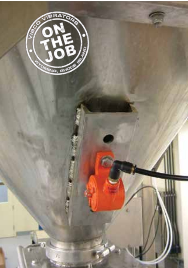
Above: Each time the hopper needs to empty, the VIBCO VS-320 Pneumatic Turbine vibrator (as seen on page 10) is activated to ensure a complete clearing of the hopper. Its walls will stay totally clean and the correct amount of material will be consistently dispensed.
