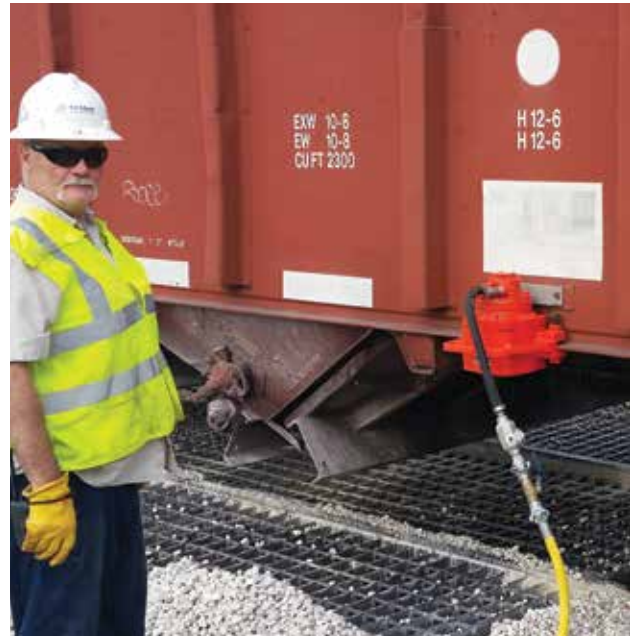
Above: A PC-3500 Big Buster (see page 34-35 and 58-59) shakes a railroad hopper car with its high force and low frequency. It easily clamps to the railcar and can be moved from place to place.
