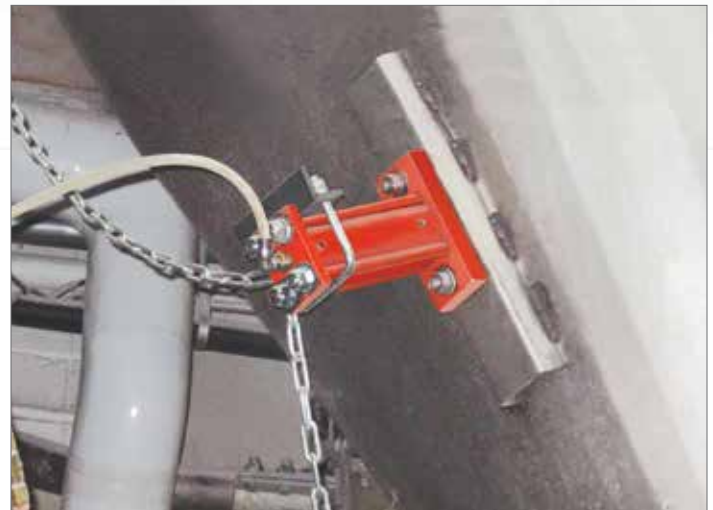
The LI Piston is used when an adjustable impact is desired to break up material bridges or ratholes.
