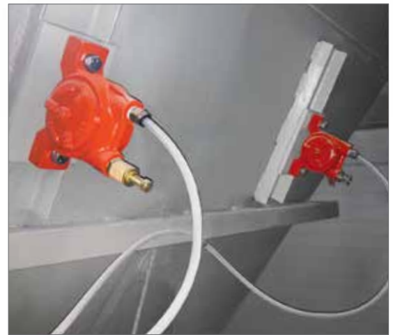
With its high force output, a BVS unit can easily move tough industrial materials in sturdy hoppers like the BVS 160 shown above. The air fitting on top helps with the flow.
