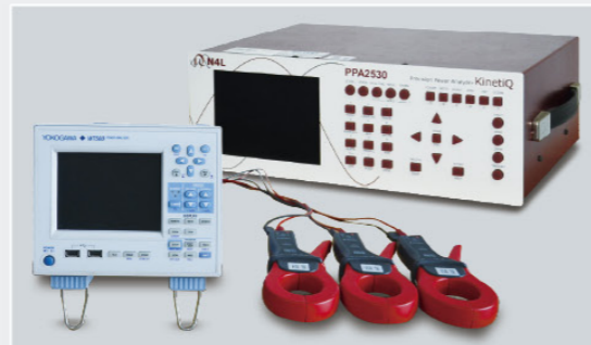
The latest multi-function and high precision electric power analyzer for AC servo system (Newtons4th Ltd,UK; YOKOGAWA, Japan)
