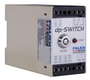
The FAUDI Aviation dp-SWITCH is designed to be connected with a mechanical dp gauge that measures the pressure difference between inlet and outlet of a filter vessel in safety-critical applications. The switching pressure is adjusted to 1 bar (15 psi) and designed to automatically stop the fuelling operation. It is suitable for competitive interchange and easy to retrofit.
