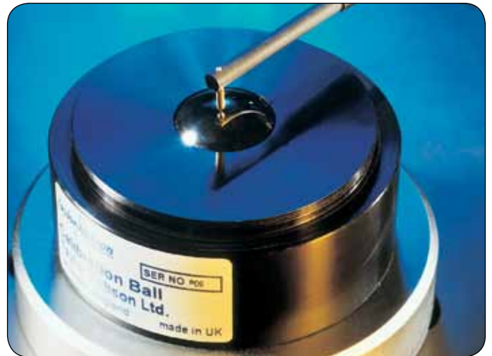
Calibration over a ball checks stylus condition, gauge range and linearity
