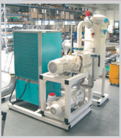
Vakuumentgasung PET-Extrusion / vacuumdegassing system for PET
